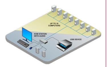
**Installation** Installing the UltraView DVI consists of connecting up to 16 DVI computer video sources to the video inputs along with their associated USB inputs and stereo audio outputs. Attach the user's monitor, keyboard and mouse, USB 2.0 peripherals, and stereo speakers to the console connectors. Apply power to the monitor and the switch, then apply power to the computers.
